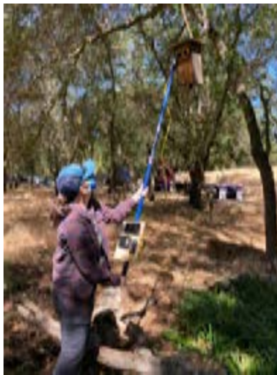
Emily Boling checks a nesting box with new device incorporating an endoscope and iPhone developed by Patrick Wagner.
